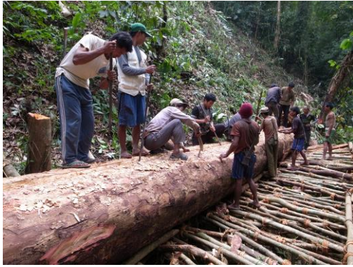
Pic 11, 12: Hollowing out the log
