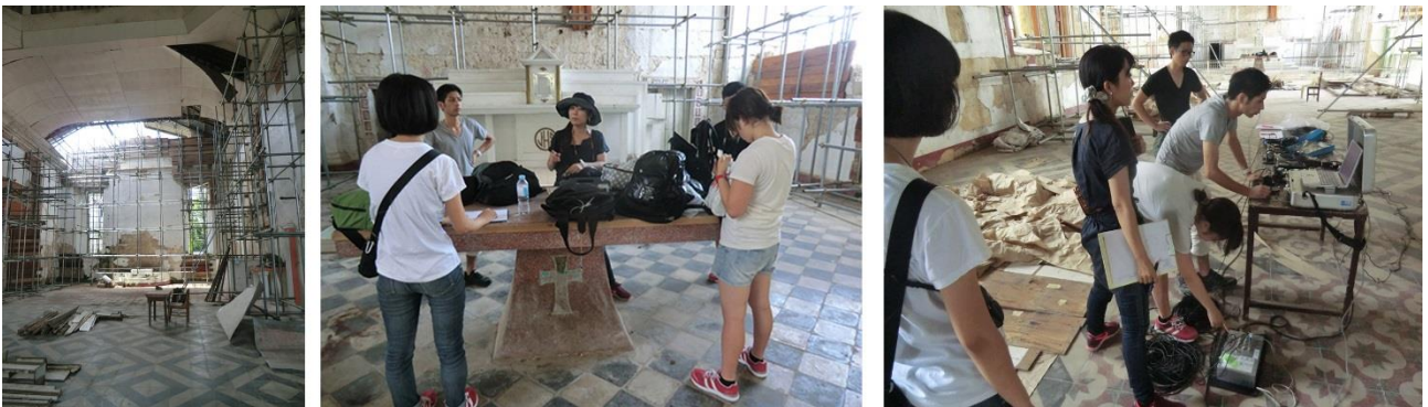
Picture 16: Microvibration measurement test on walls of Cortes church, Bohol island
