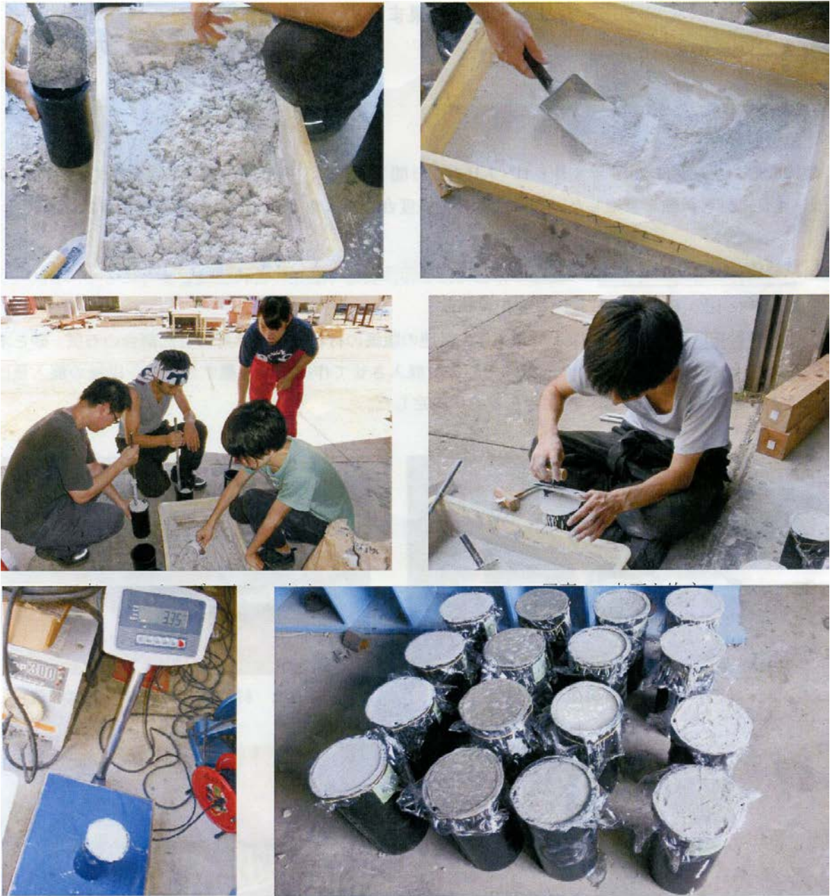
Picture 3. Construction of traditional mortar cylinder in Tokyo metropolitan University
